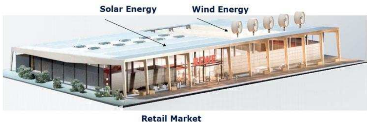
Figure 4 Proposed building integrated power system
